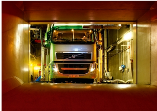
Figure 1.3: A commercial vehicle prepared for thermal performance testing in a climatic wind tunnel.
