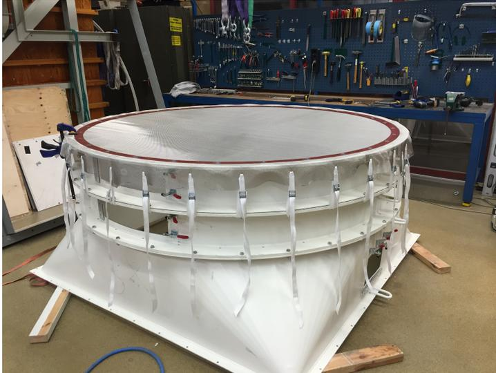
Figure A.1: *Metallic screen mounting. "High tec" pretension system.*
