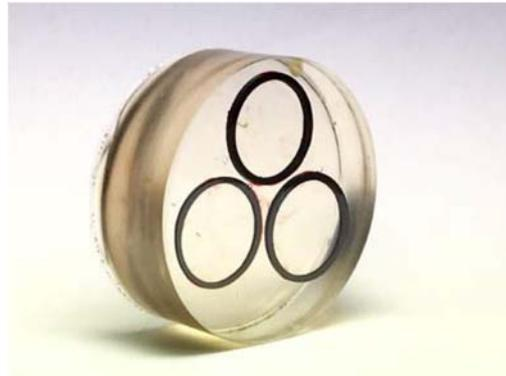
**Figure 1.** Microscopy samples in epoxy casting.
