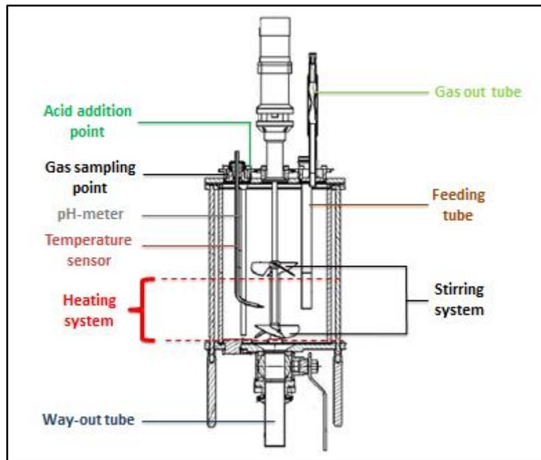
Figure 1: Reactor scheme
