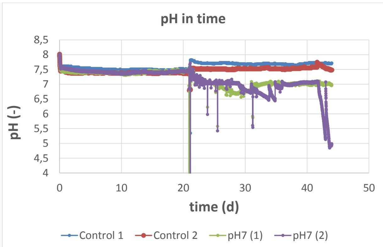
Figure 7: Cumulative gas production and pH of reactors; GB1 & GB2 were pH controlled at 7.0 while GA1 & GA2 were under standard conditions (control)
