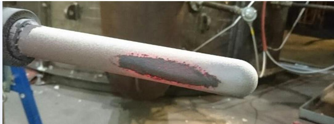
**Figure 7. Top panel:** Schematic of the probe showing how the thermocouple is protected by ceramics. Courtesy of Adrian Gunnarsson [69]. **Bottom panel:** Photograph of the protective ceramic around the thermocouple. The gas inlet is on the other side and is therefore not visible in this shot. Hot coal particles adhere to the ceramics after the measurements.
