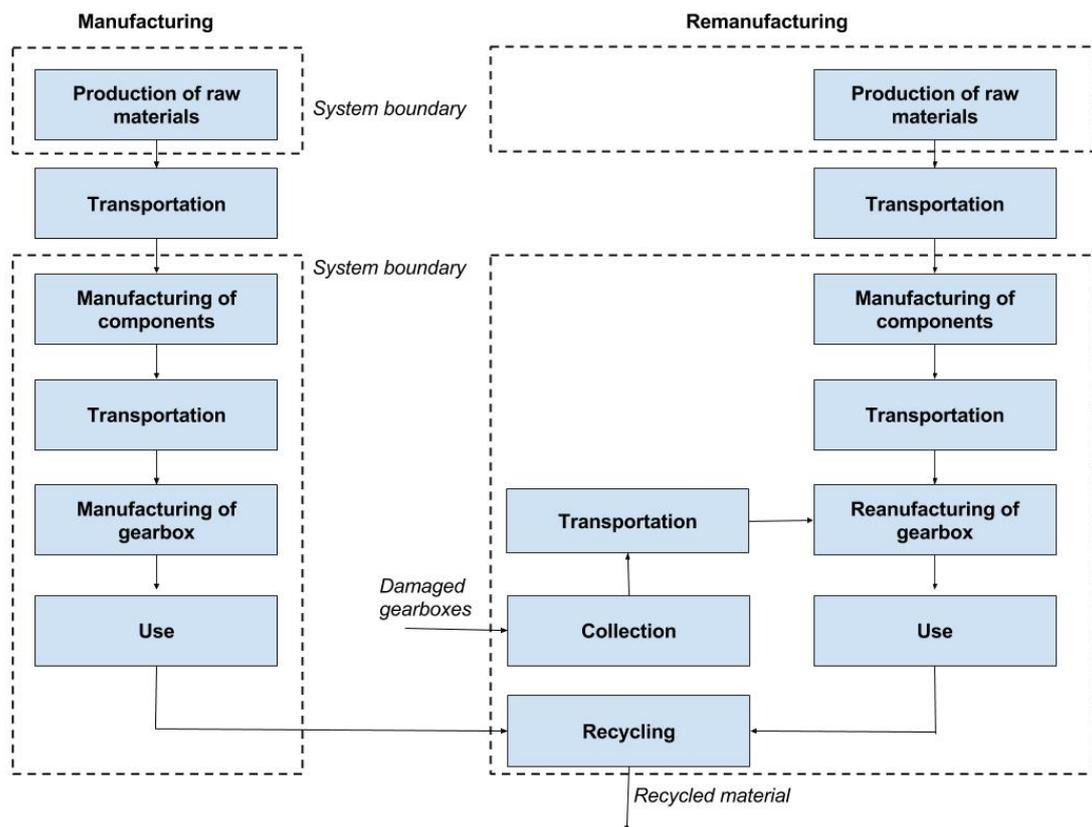
**Figure 5.1:** Initial flow chart showing the life cycle and natural boundaries of both new and remanufactured gearbox.
