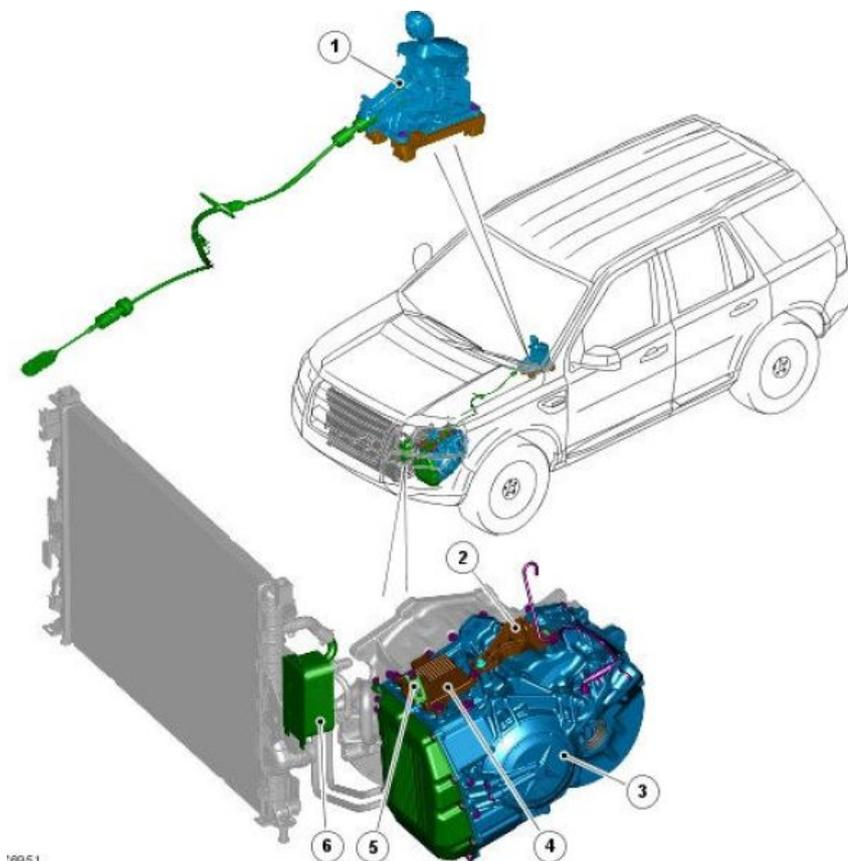
Figure 3.1: Location of the gearbox in a car [29].
