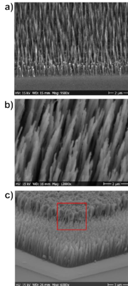
Figure 2: a) CNFs as grown; b) CNF coated with dielectrics; and c) Integrated 3D capacitor.
