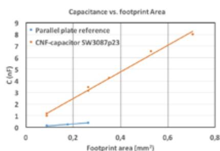
**Figure 3:** Comparison of Smoltek's solid-state initial integrated capacitor prototype (SmolCACH™) and parallel capacitors.
