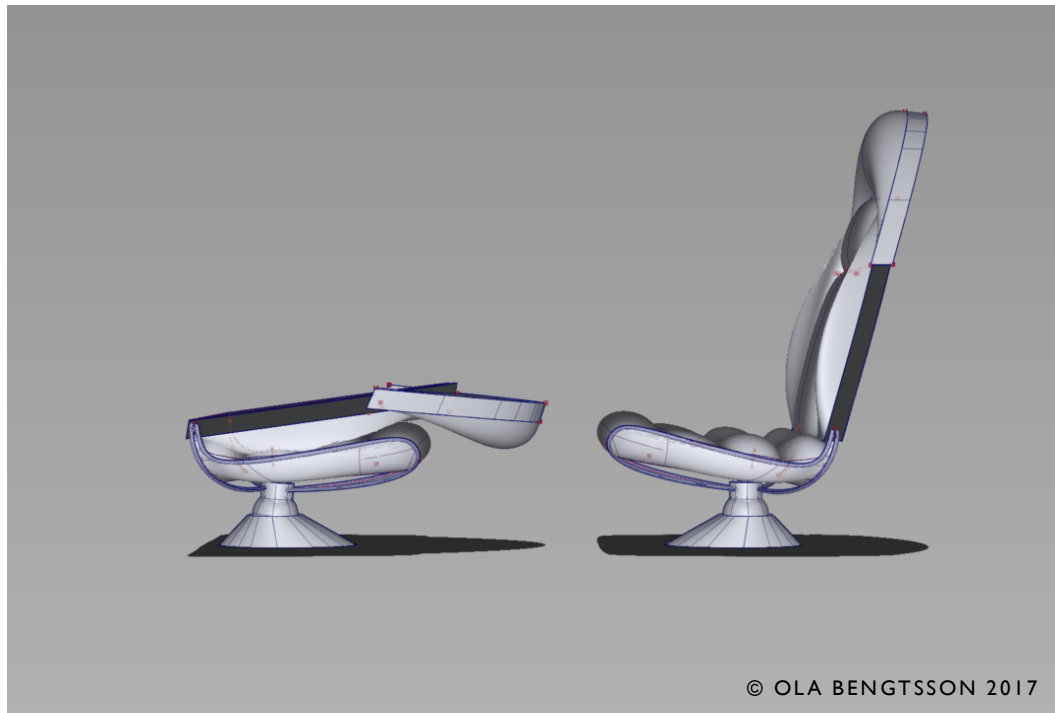
Figure 37: Concept with a seat transforming into a footrest.
