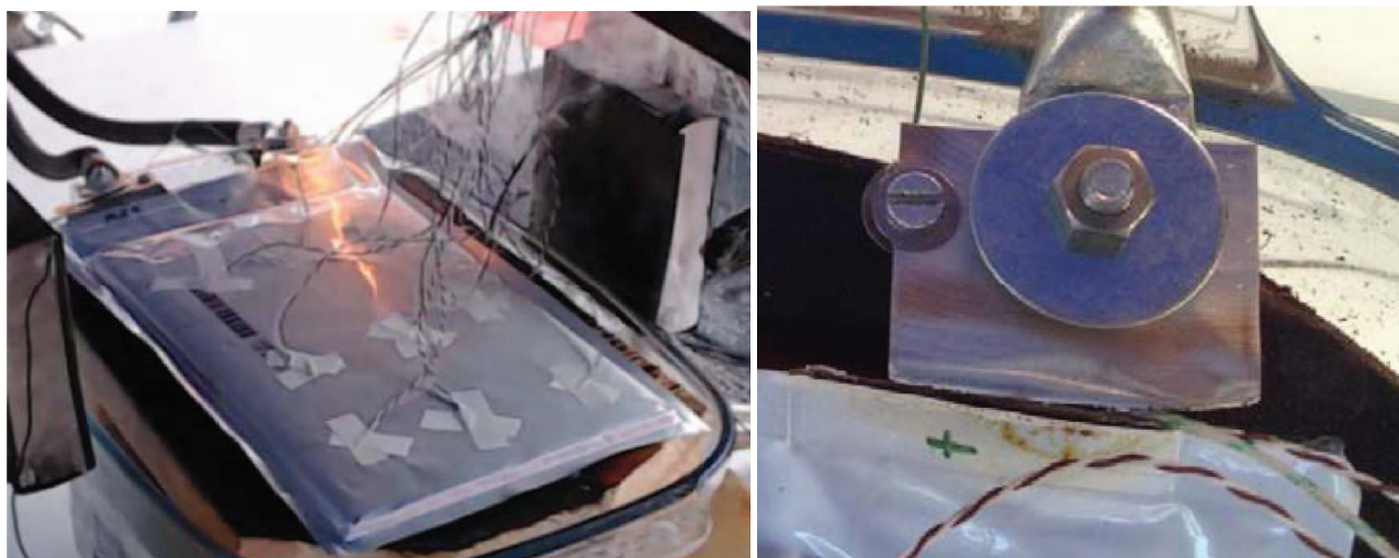
Figure 13. Short circuit of European Batteries cell, photo (left) showing the flame and smoke from the burnt off positive terminal tab, the photo (right) after the test shows the burnt off tab.
