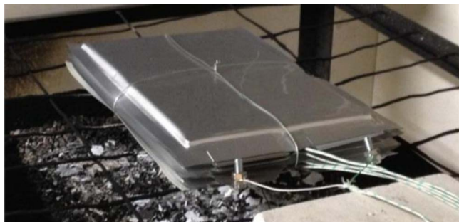
Figure 2. Photo of 5-cell-pack placed on wire-gratings.
