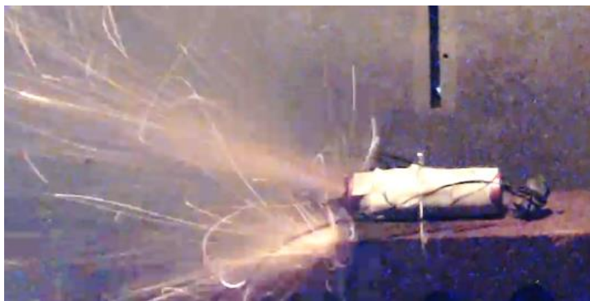
Figure 6. A commercial Li-ion cell of type 18650 undergoing thermal runaway in external heating abuse test.
