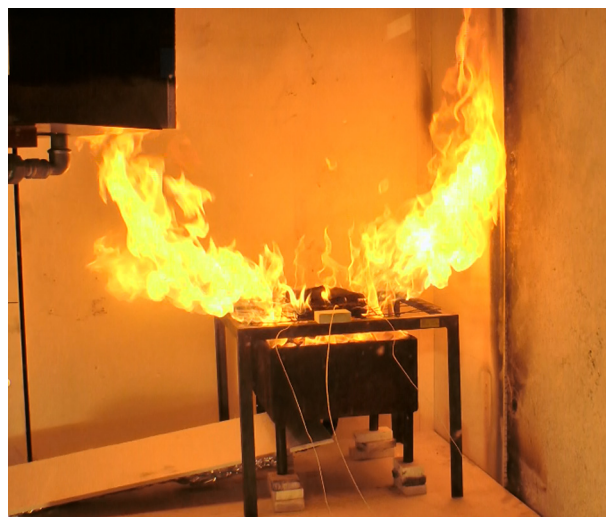
Fig. 6. Outbursts from EiG 100% SOC (test 1).
