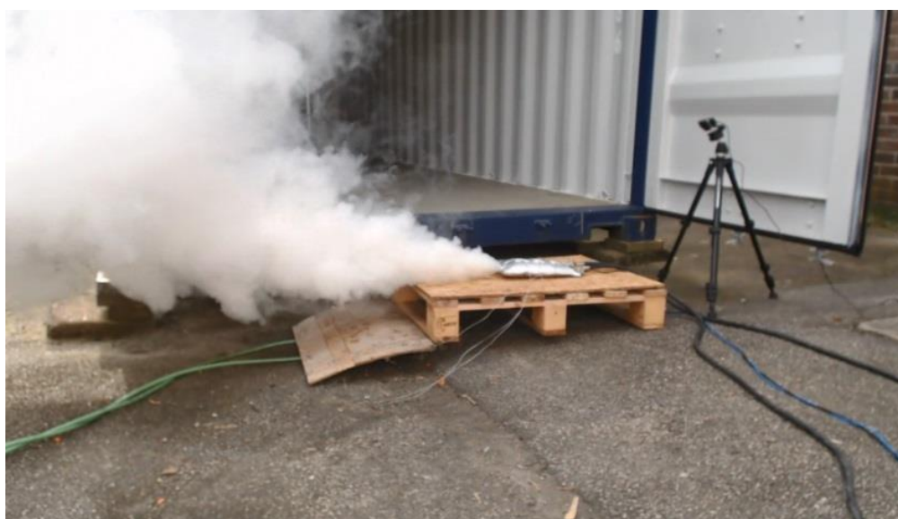
Figure 45. Gas release before fire upon overcharge abuse with a 2 C-rate current of a 30 Ah cell with LATP/NCA.
