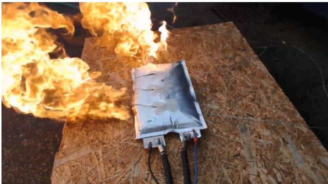
Figure 42. Overcharge abuse with a 2 C-rate current of a 30 Ah cell with LATP/NCA during fire caused by the abuse.
