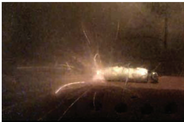
Figure 4. Samsung 18650 cell at the beginning of thermal runaway releasing ignited material.
