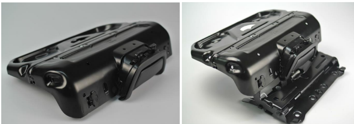
Figure 8. Folding mechanism of the integrated booster cushion [49].
