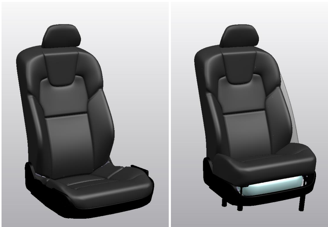
Figure 45. The ICSC in uninstalled position (adult seat) and installed position (child seat). The seat cushion in the uninstalled position consist of two sections and the installed position consist of one section.
