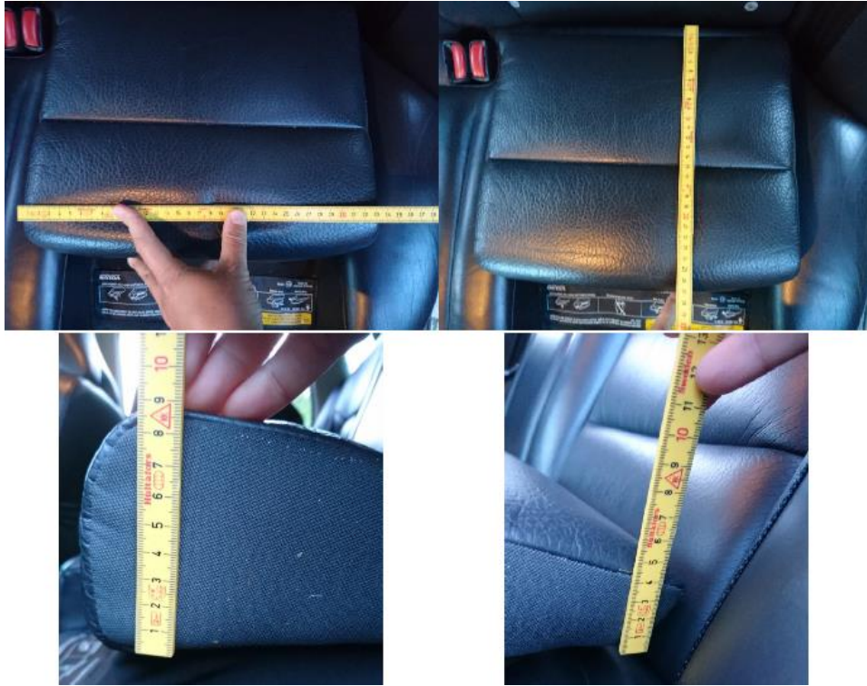
Figure 7. Measurements of an integrated booster cushion.
