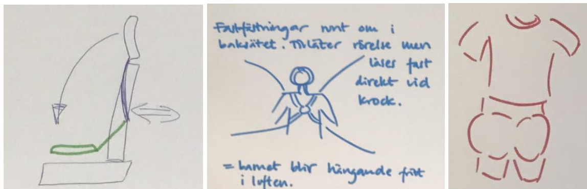
Figure 30. Innovative suggestions. To the left, neck support is folded down. In the middle, the belt enables the child to move freely in the rear seat. To the right, Boosting pants that the child wears to be raised to fitting height.
