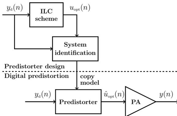
**Figure 5.6.** Block diagram of the iterative learning control based digital predistortion technique. In this technique, the ILC scheme described in Chapter 3 is first used on the power amplifier to identify the optimal predistorted signal  $u_{\text{opt}}(n)$  that drives the PA to the desired linear output response  $y_d(n)$ . After that,  $y_d(n)$  and  $u_{\text{opt}}(n)$  are used to identify a predistorter model.
