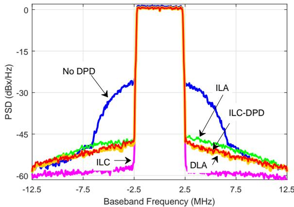
**Figure 5.8.** Power spectral density (PSD) of the measured PA output signal obtained without DPD, and after applying ILC, ILA, model-based DLA, and ILC-DPD for a Class B PA driven under high compression.
