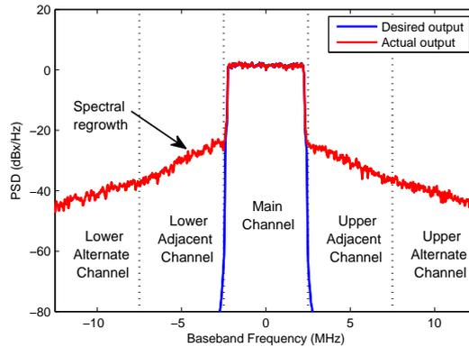
**Figure 1.1.** Spectra of the output signal of a Class AB power amplifier driven with a 5 MHz-LTE signal. Note that due to the nonlinearity of the PA, spectral regrowth is generated in the neighboring channels.
