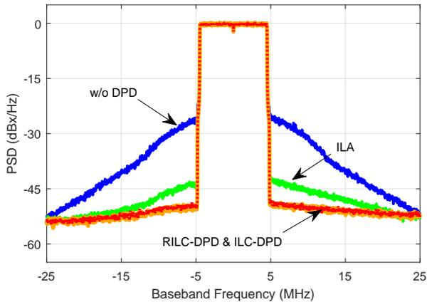
**Figure 5.10.** Spectrum of the PA output signal obtained without DPD and after using the proposed RILC-DPD, the conventional complex-valued ILC-DPD, and ILA. Note that the spectrum of the output signals obtained with RILC-DPD and ILC-DPD overlap each other.
