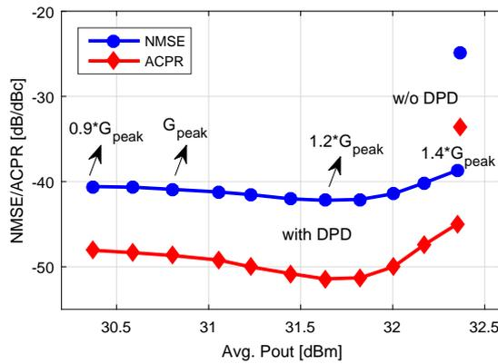
**Figure 5.2.** NMSE and ACPR results versus average output power obtained using different normalization gain values. Note that the use of different normalization gain values produce output signal with different average powers.
