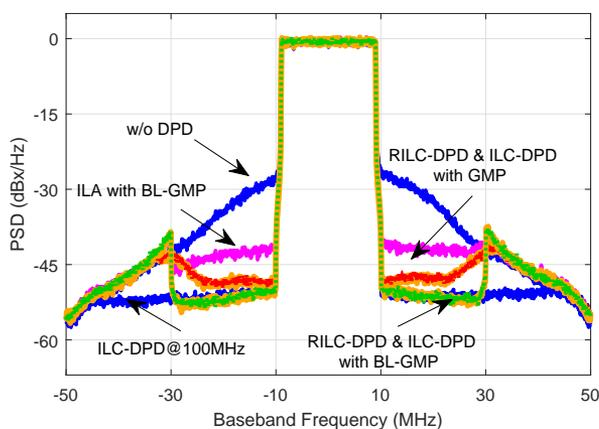
**Figure 5.11.** Spectrum of the measured output signal obtained without DPD and after using the proposed RILC-DPD, ILC-DPD, and ILA with a linearization bandwidth of 60 MHz and GMP and band-limited (BL)-GMP models. For reference the spectrum of the output signal after using ILC-DPD with a linearization bandwidth of 100 MHz. Note that RILC-DPD with a BL-GMP model provide similar spectral leakage reduction as ILC-DPD with a linearization bandwidth of 100MHz.
