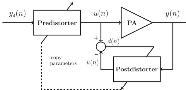
**Figure 5.3.** Proposed variant to the indirect learning architecture. Unlike the conventional indirect learning architecture, this variant eliminates the normalization gain and uses the desired PA output response as input to the predistorter.
