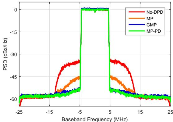
**Figure 4.1.** Power spectral density (PSD) of the output signal obtained before and after the PA was linearized with a memory polynomial (MP) model, a generalized memory polynomial (GMP) model and a memory polynomial based predistorter (MP-PD) model .
