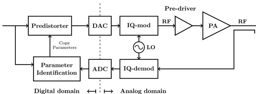
**Figure 3.2.** Block diagram of a digital predistortion system
