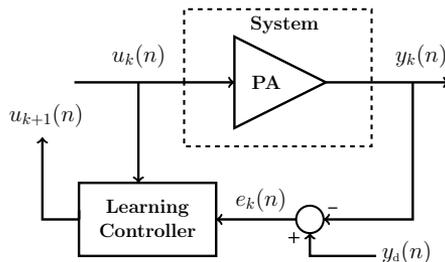
**Figure 3.4.** Iterative learning control scheme for the linearization of power amplifiers.
