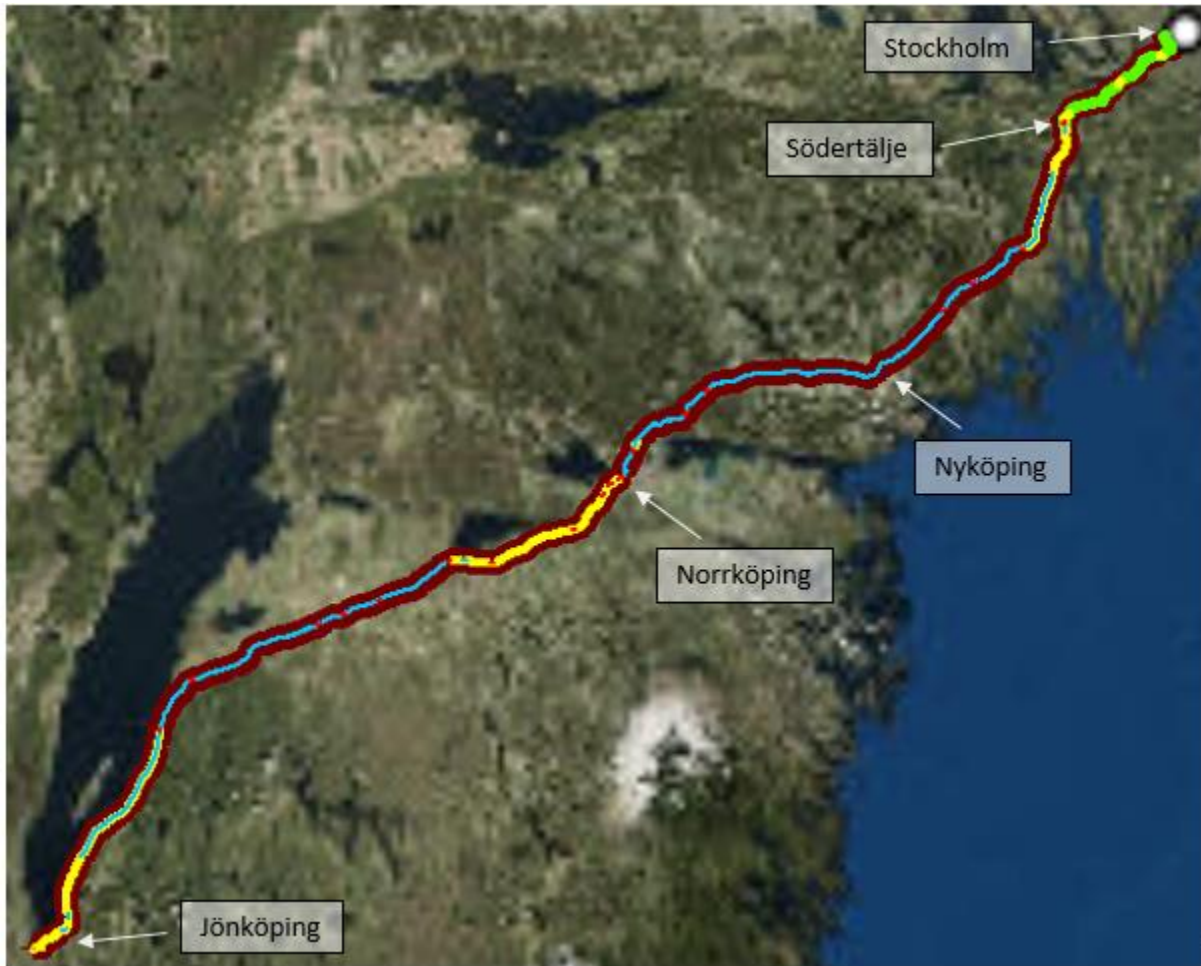
Figure 23. Route E4 between Stockholm-Jönköping with road segments color coded according to group belonging for heavy vehicles.
