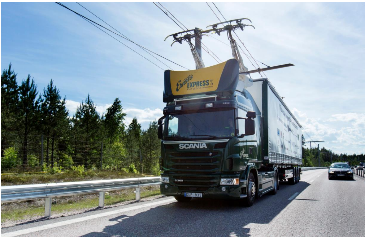
Figure 5. A hybrid G360 4x2 Scania lorry utilizing electrical energy from the conductive overhead line ERS solution at Sandviken, Sweden (Scania, 2016).
