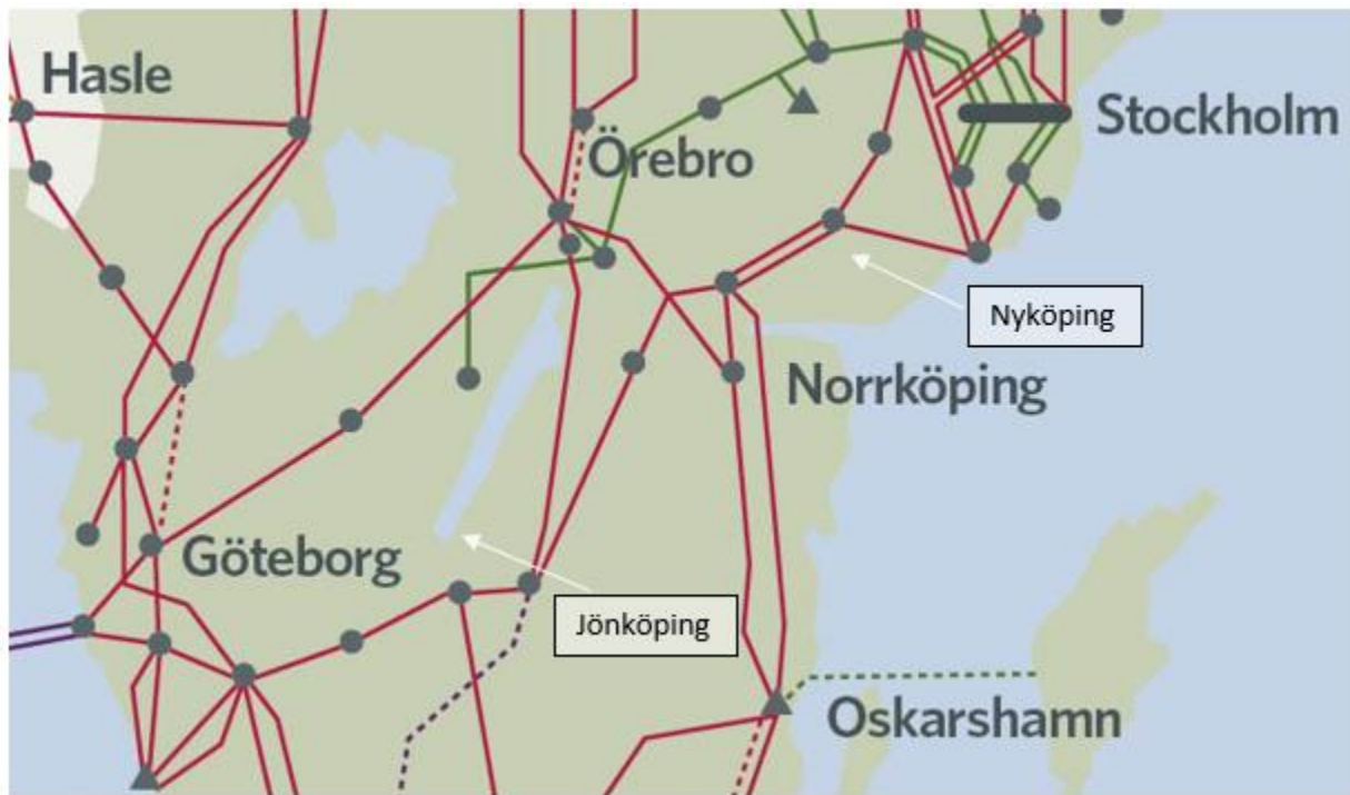
Figure 7. Map over the national electricity grid in southern Sweden (SVK, 2016). Red lines correspond to a 400 kV voltage level, green to a 220 kV voltage level.
