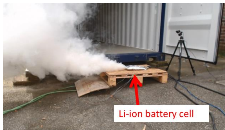
Figure 8 Gas release (venting) during overcharge abuse from a 30 Ah Li-ion battery cell with pouch prismatic packaging. Photograph: Fredrik Larsson.
