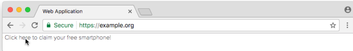
Figure 7.2: Example of removing the link as visual feedback for blocked navigation
