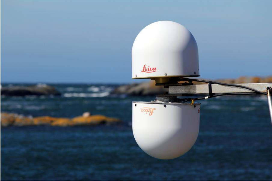
Figure 1.2: *The GTGU/GTGD research installation at the Onsala Space Observatory, Sweden, consisting of two permanently operating antenna/receiver pairs.*
