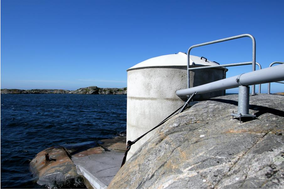
Figure 1.3: *The Super Mareograph at the Onsala Space Observatory. Inside the stilling well there are four instruments — two pressure sensors, one radar, and one laser — measuring the water level continuously. A third pressure sensor is mounted outside the well.*
