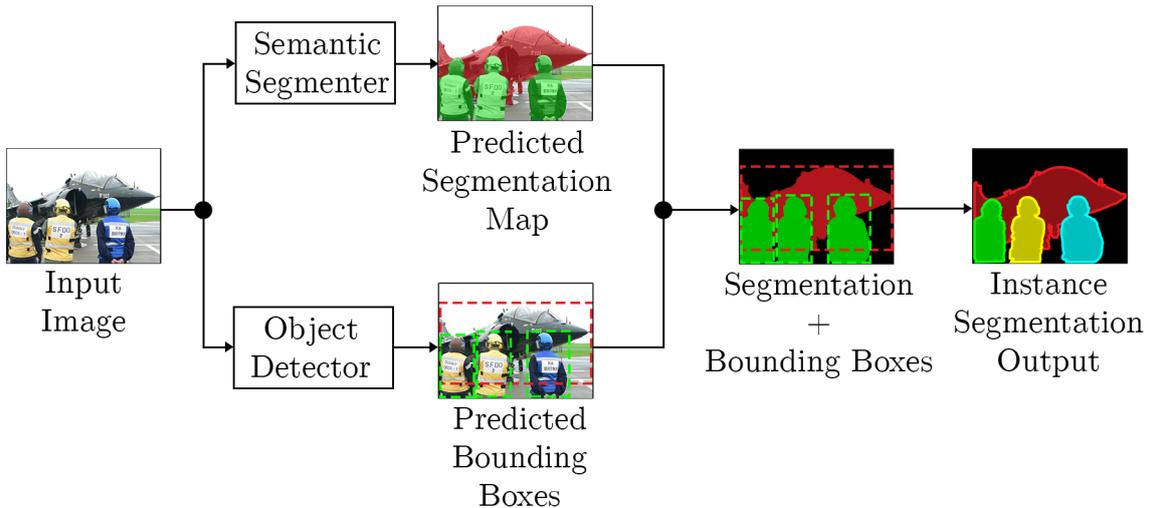
**Figure 3.1:** Functioning of the naive approach to instance segmentation.
