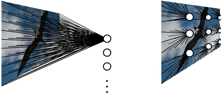
(a) Fully connected layers, used in regular neural networks.
