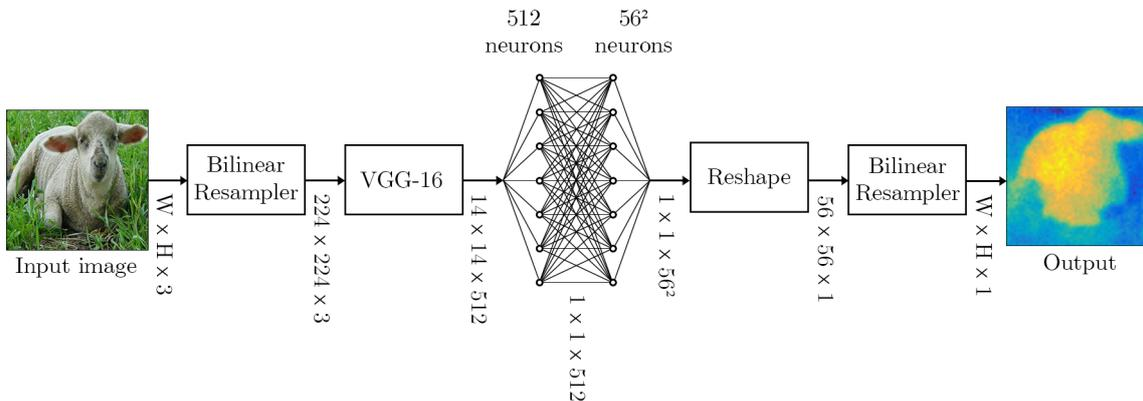
**Figure 3.7:** DeepMask architecture. “VGG-16” is the altered version of the VGG-16 CNN, as mentioned in the text. The vertical text between each layer demonstrates the size of the data in that step, and the “Output” subimage is a heatmap illustrating the mask scores (yellow means high probability of being part of the mask, while blue means low).
