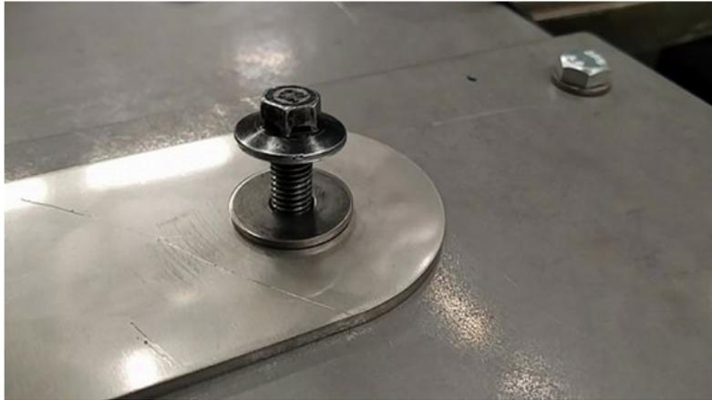
**Figure 4.6:** Small washer between the bolt and the component.
