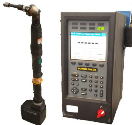
**Figure 3.3:** The tool with 800RPM and the Power Focus controller.
