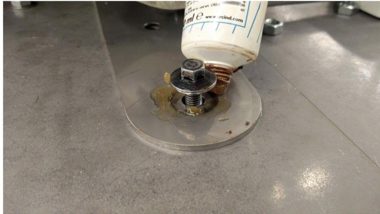
**Figure 4.8:** Oil between bolt head and component.
