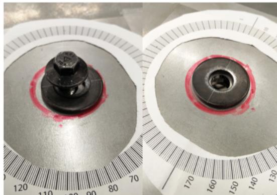
**Figure 4.18:** To the left; Washer off center. To the right; Washer in center.
