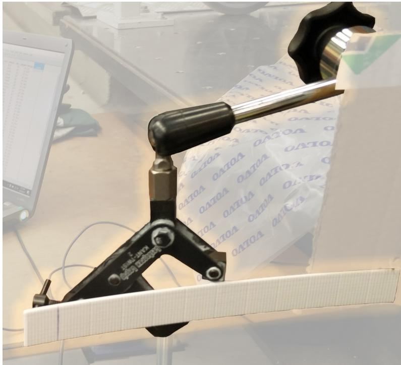
**Figure 4.21:** The protractor that was used for measuring the rotation of the component, held up by a mechanical arm. The radius of the protractors arc was 1000 mm and could measure up to 10 degrees.
