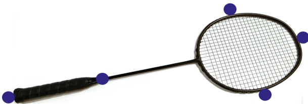
Figure 3.5: Markers used in the motion capture. Attached on the outside of the frame and handle.
