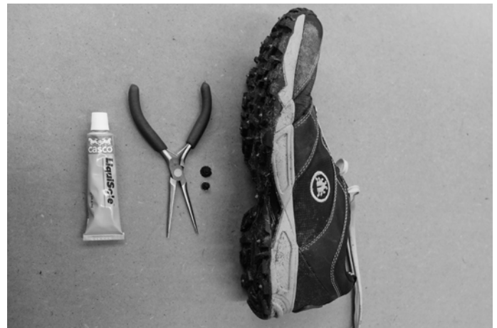
Figure 8. Tools needed for the replacing of a stud.
