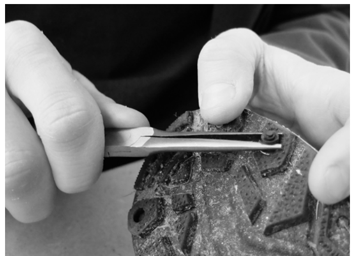
Figure 10. Placing the stud in the cavity in the sole.
