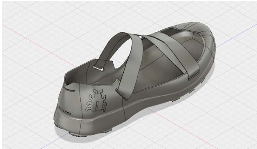
Figure 76. Concept shoe in fusion 360, high heel counter.
