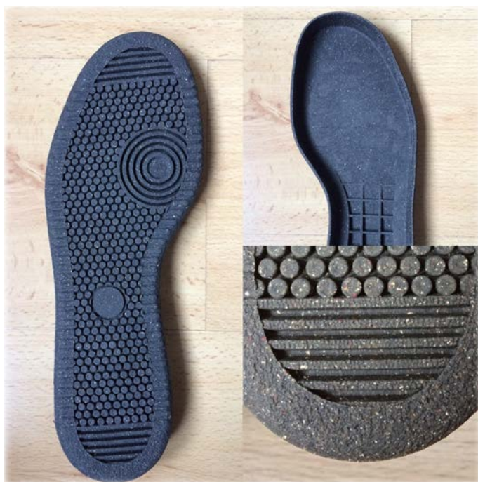
Figure 34. Sole produced from recyclates from old shoes (SOEX Footwear Recycling, 2016, C).
