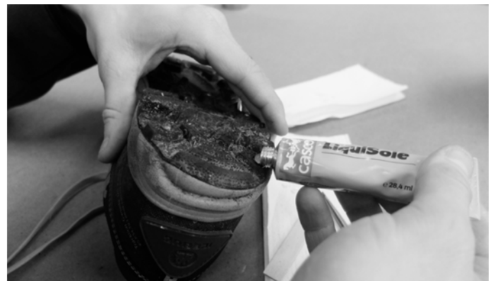
Figure 9. Adding glue in the sole cavity where the stud should be placed.
