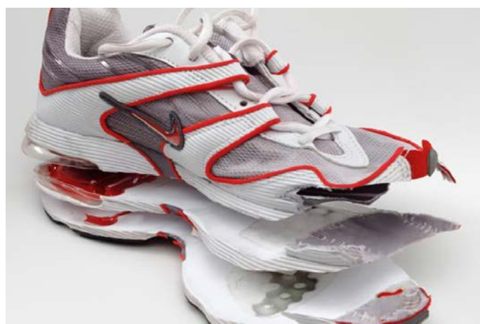
Figure 32. A Nike shoe that have been sliced in preparation for it to be grinded (Nike, 2016).
