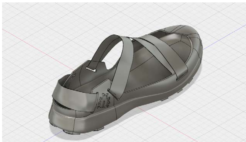
Figure 78. Concept shoe in fusion 360, low heel counter with webbing.
