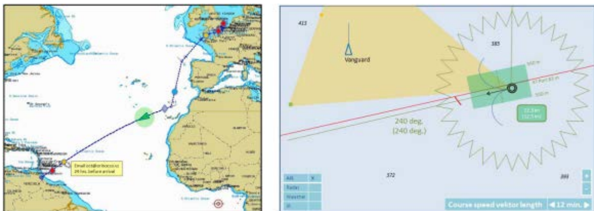
Picture 3: Spatial Overview, ECDIS screen providing information of the vessel and with AIS targets, the route plan is also shown. Picture: MUNIN
