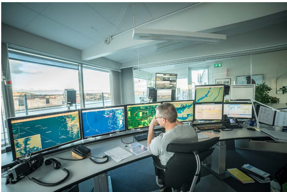
Picture 8: Vessel Traffic Service with multiple screens providing AIS and RADAR information of the entire Port of Gothenburg
