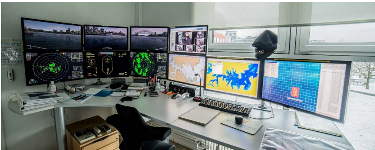
Picture 1: Chalmers Simulator Instructor System, with a screen with an overview of the area on the right and multiple screens on the left that shows the students instruments, possibility of switching screens between multiple simulator bridges.
