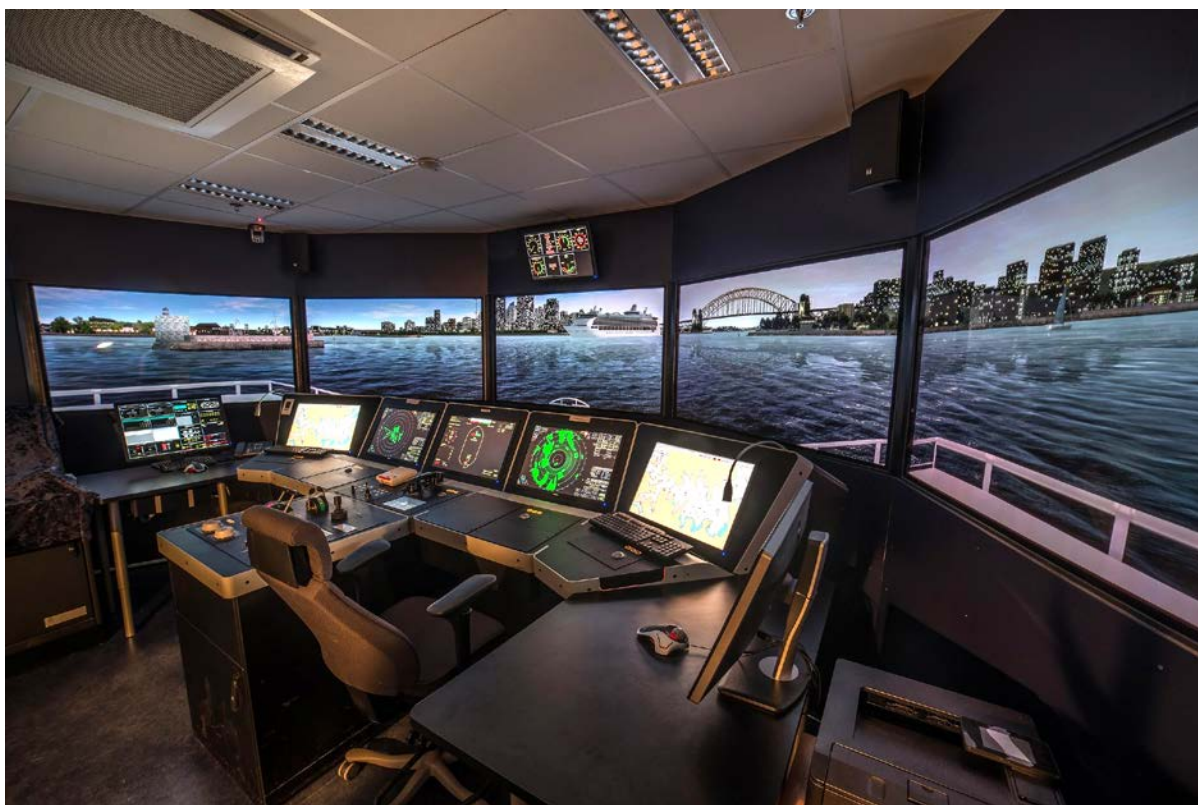
Picture 7: Chalmers Simulator Bridge with RADAR, ECDIS and conning screens. This is how a Situation Room could look like, with camera-feeds from the ship or a 3D generated picture.
