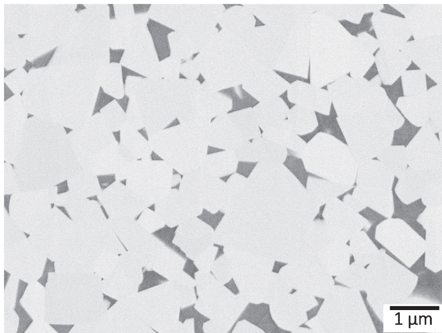
Figure 3: The general microstructure of WC-Co seen in cross-section with an interconnected skeleton of WC grains (bright) and Co-binder (dark) in-between.
