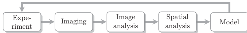
Figure 1.1: Workflow from experiments with images to 3D models: Materials are experimentally prepared and imaged using electron or laser microscopy. The images are processed in an image analysis routine and methods from spatial statistics are used to characterize and model the material structure. Conclusions drawn from the model can provide valuable input for further experiments.
