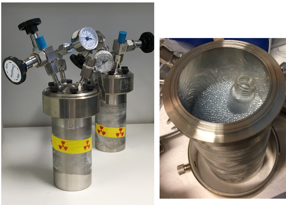
Figure 5. Assembled autoclaves (left picture). Inside of autoclave for homogeneous radiolysis experiment, including vial for ^{238}\text{Pu} solution and glass beads for volume reduction (right picture).
