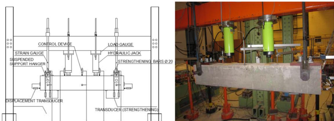
Figure 1 – Photo and drawing of the indirectly supported four-point bending test.
