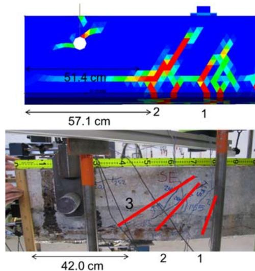
Figure 4 – Comparison of the crack pattern for the beam M4; the remaining anchorage length is given in cm.
