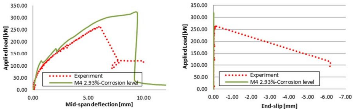
Figure 3 – Results of 3D FE analysis in comparison with the experiment.
