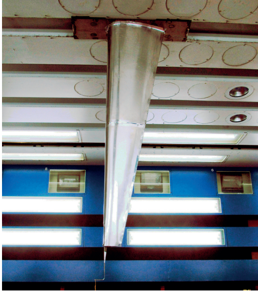
Figure 3.1: Prandtl tube mounted on custom built wing used for measurements of the longitudinal pressure distribution.
