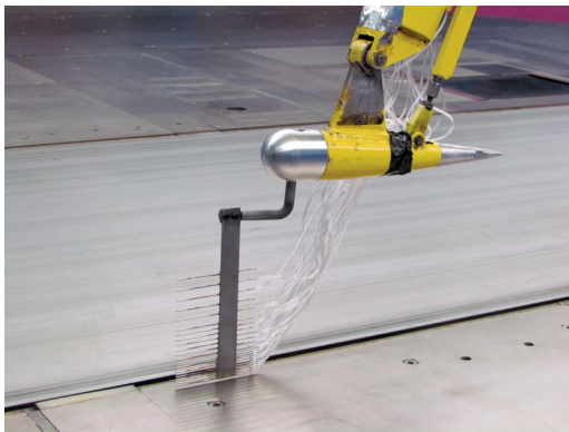
Figure 3.2: Boundary layer rake mounted on the traversing gear [2].
