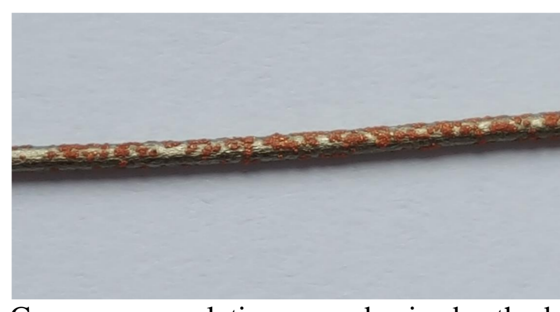
Copper accumulation on undersized cathode
