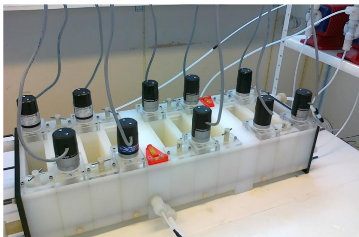
Fig. 39. A sample of mixer-settler system for copper and zinc extraction from MSWI fly ash leachate.
