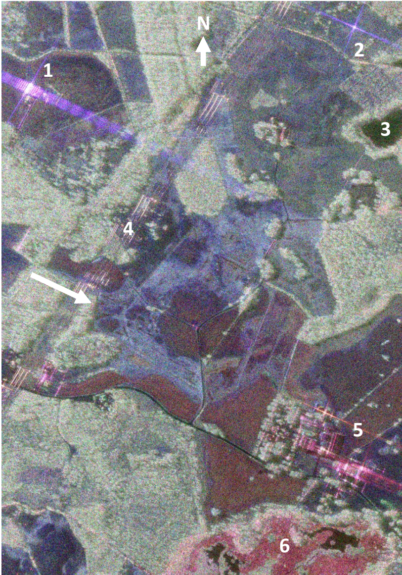
Figure 2.5: Geocoded L-band SAR image from Remningstorp in the south of Sweden. Acquired with SEHTI as part of the BioSAR 3 campaign using a bandwidth of 150 MHz at 1.3 GHz. Resolution is 0.9 m by 0.9 m. Polarimetric information is included by the use of the Pauli decomposition for the RGB channels: HH-VV (even-bounce), HV (volume scattering), HH+VV (odd-bounce). Courtesy: ONERA.
