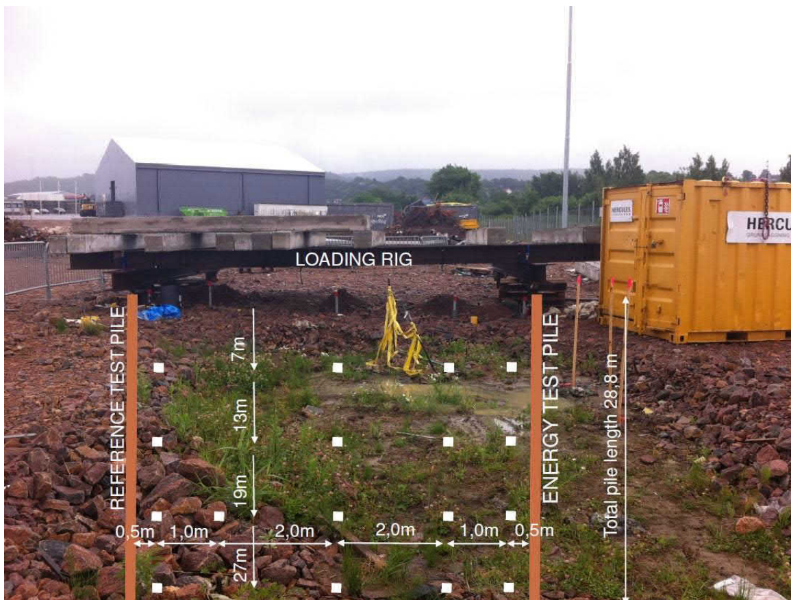
Figure 3. Utby test site. Position of sensors (BAT) in the ground for logging of temperature and pore pressure in the soil.
