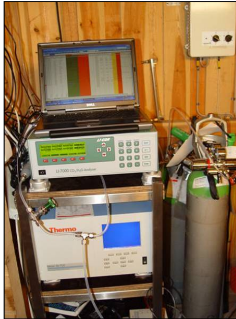
Figure 34. The Sniffer system measuring \text{SO}_2 and \text{CO}_2 is shown together with calibration bottles.
