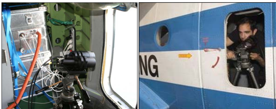
Figure 17. The optical system measuring \text{SO}_2 and \text{NO}_2 in the reflected solar light.
