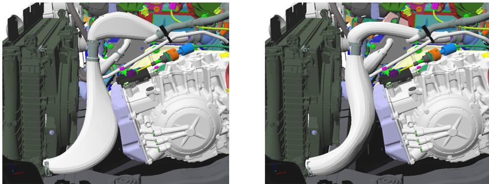
(a) Tolerance envelope with respect to a length tolerance of  $\pm 50mm$  on each hose.
