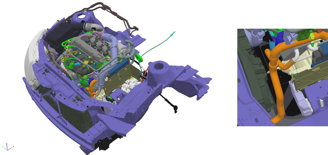
Figure 3.1: Cooler hoses in the engine compartment of a car.
