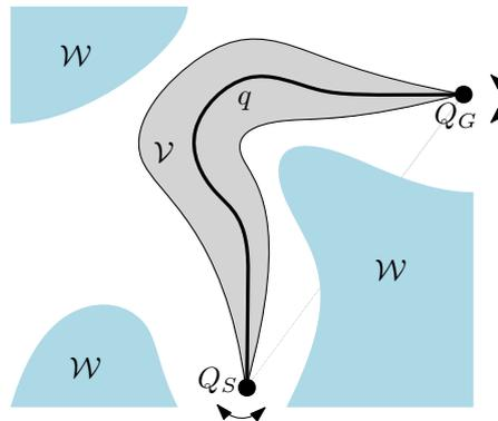
Figure 3.6: A tolerance envelope of a D1O with respect to rotational fixture tolerances at grip points  $Q_S$  and  $Q_G$ .
