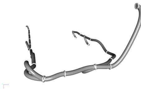
Figure 2.2: A wiring harness modelled as a deformable 1D system.
