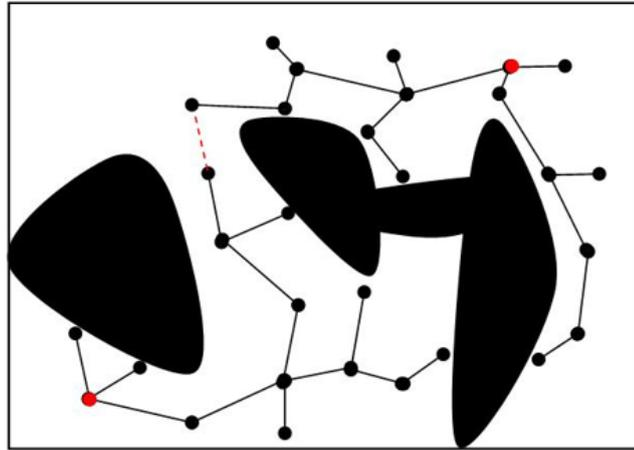
Figure 2.3: A probabilistic roadmap over a 2D configuration space.
