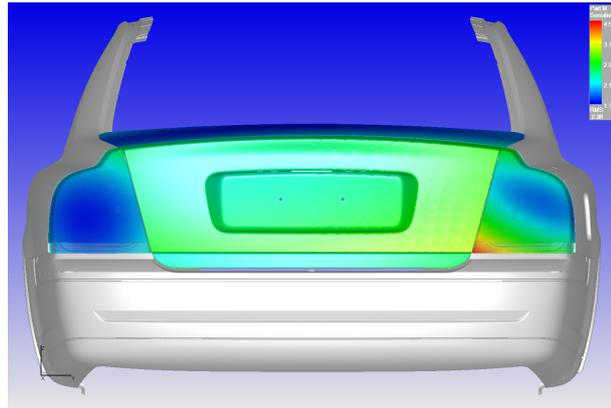
Figure 2.5: Color-coding of sensitivity in a rigid assembly.
