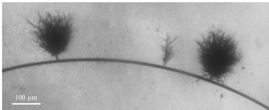
**Figure 3**, Electrical trees in polyethylene grown from a 10 µm thick wire.
