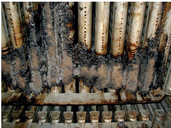
*Figure 1.2. Example of scaling in a black liquor evaporator. Courtesy of Valmet (2015).*
