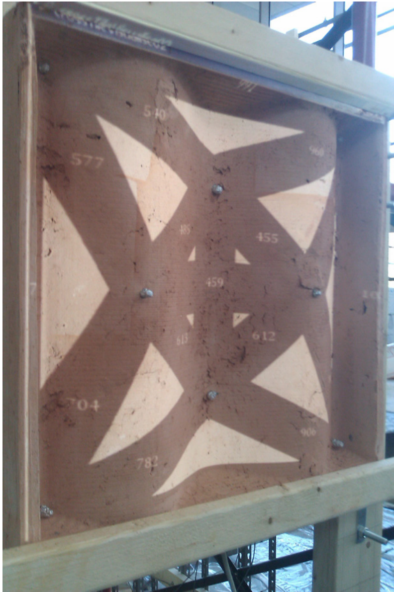
Figure 11. 'Sensor active clay tile' is a ceramic tile that can be used as a sensor by measuring the internal resistance of the material. Electrodes are drilled into the material, and in turn, current is sent from each electrode to every other, while resistance is measured. A projection on the material itself shows the resistance value between each electrode. As the humidity in the material changes, the internal resistance changes respectively.
