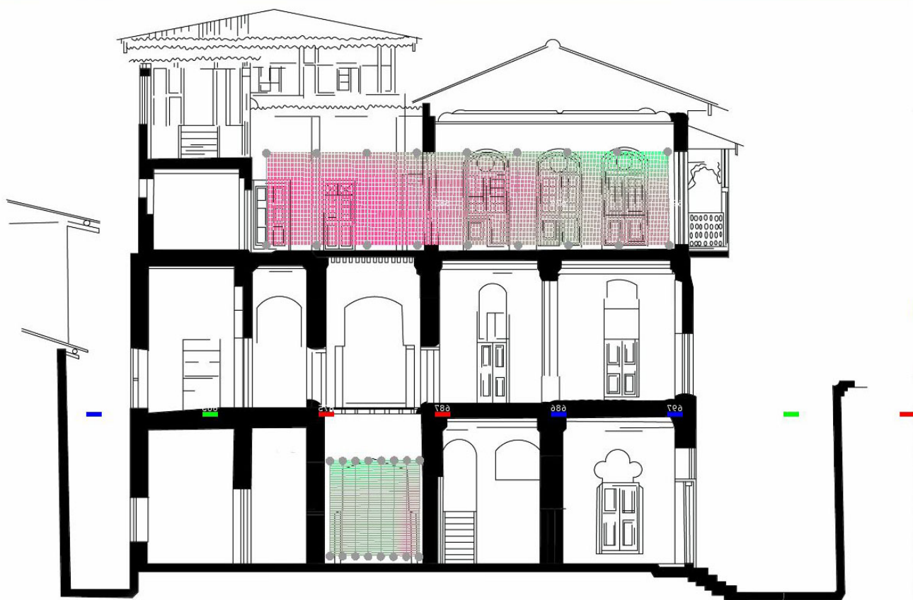
Figure 33. The refurbished house where the central shaft is blocked, resulting in lack of airflow on the lower levels.
