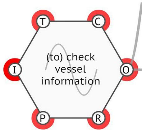
Figure 6. Example of a FRAM function, '(to) check vessel information'.
