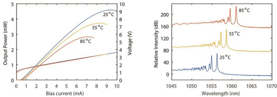
**Fig.2** Left: Output power and voltage vs. current at 25, 55, and 85°C. Right: Emission spectra at 4 mA.
