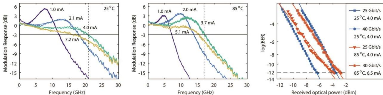
**Fig.3** Left and middle: Small signal modulation response at 25 and 85°C. Right: Data transmission at 25 and 40 Gbit/s at 25°C and 25 and 30 Gbit/s at 85°C.
