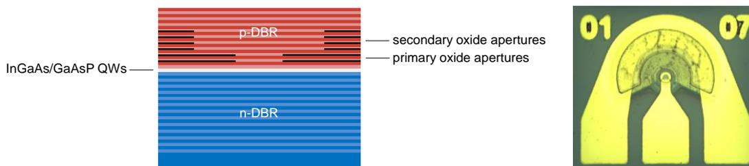
**Fig.1** Left: VCSEL design with multiple oxide apertures and strained InGaAs/GaAsP QWs. Right: Microscope image of a fabricated VCSEL.
