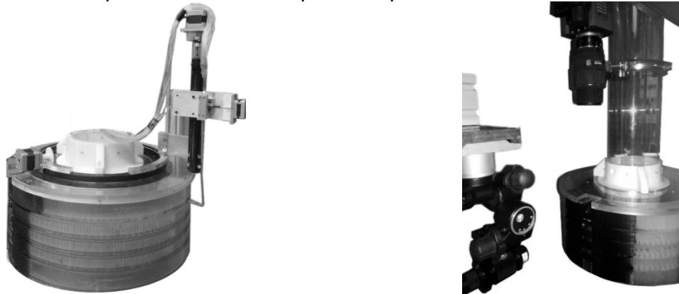
(a) Total pressure rake on a three-axis traversing (b) 2D PIV configuration
