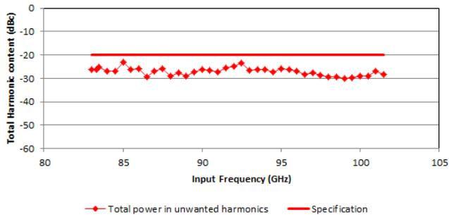
Fig. 7. Measured total power of the unwanted harmonics (x3 and above) at the output of the doubler WR5.1x2.
