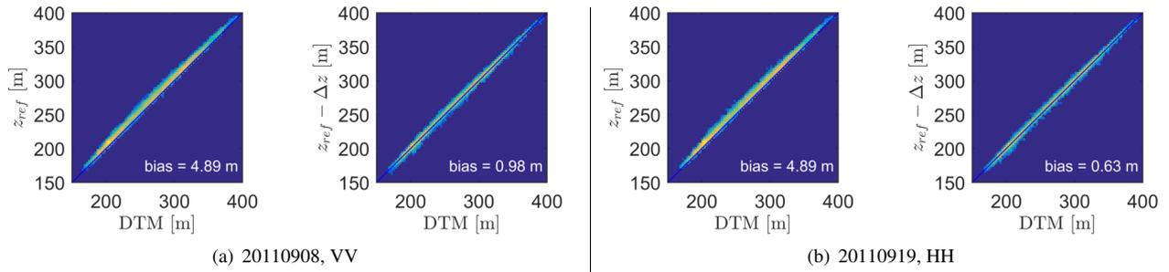
**Figure 4:** Scatter plots showing the improvement of ground topography mapping after correction of  $z_{ref}$  with  $\Delta z$  estimated from TLM inversion. As reference height  $z_{ref}$ , DEM obtained from the bistatic pair was used. Measured bias is shown, computed as the average difference between estimate and reference.
