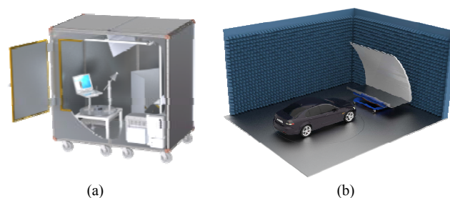
Fig. 2 (a) Drawing of Bluetest's RTS60 reverberation chamber for OTA characterization and testing of antennas and devices in RIMP. (b) Drawing of the OTA testing environment in semi-anechoic chamber in Random-LOS [6]
