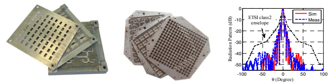
Fig. 1. 8x8 and 16x16 slot arrays with gap waveguide distribution networks for V-band (60 GHz) consisting of three metal layers, and simulated and measured radiation patterns of the larger 16x16 slot version.
