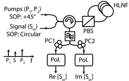
**Fig. 1:** Schematic for quadrature decomposition based on a polarization-assisted phase-sensitive processor with a polarization-diverse implementation.
