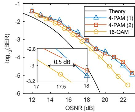
**Fig. 4:** BER vs. OSNR for the 16-QAM signal and both quadrature demultiplexed 4-PAM signals.
