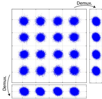
**Fig. 3:** Constellation diagrams of the incoming 16-QAM signal and the two quadrature demultiplexed 4-PAM signals.
