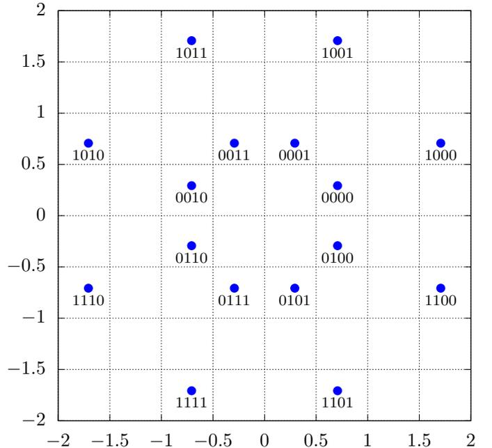
Figure 17: Joint mapping for two QPSK constellations.
