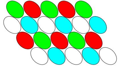
Figure 2: 4-color frequency reuse scheme.
