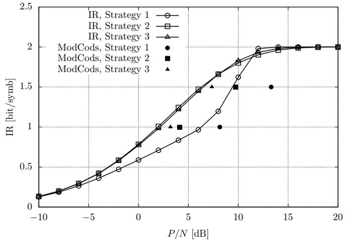
Figure 14: IR and ModCods of “User 1” in case 1. ModCods are based on DVB-S2 LDPC codes.
