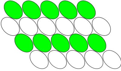
Figure 3: 2-color frequency reuse scheme.
