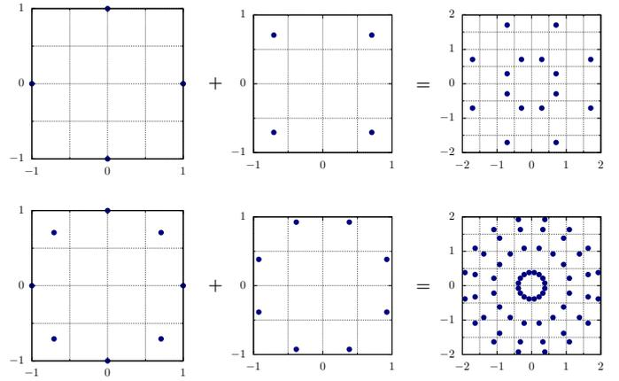
Figure 16: Joint constellations resulting from two QPSK (top) and from two 8PSK (bottom) constellations.
