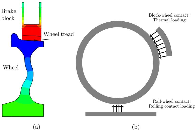
Figure 1.1: Schematic diagram of wheel, block and rail subjected to combined thermal and contact loading.
