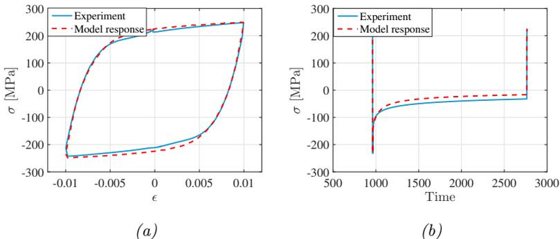
Figure 2.1: Modelling of cyclic and viscous phenomena at 600 °C for 1 % strain amplitude (a) stress vs strain for the cycle before the hold time (captured by the hardening variables) and (b) relaxation behaviour captured by the overstress function and the static recovery.
