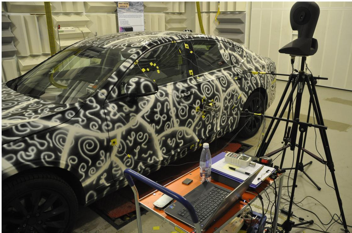
Figure 3.2.: Measurement setup using accelerometers and an artificial head microphone.
