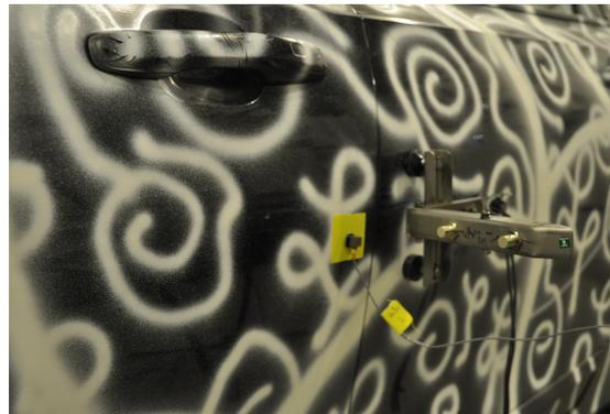
Figure 3.6.: Magnetic velocity sensor applied during the classical approach.
