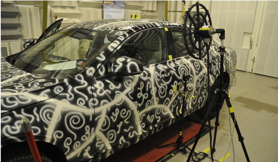
Figure 3.1.: Measurement setup using an acoustic camera.
