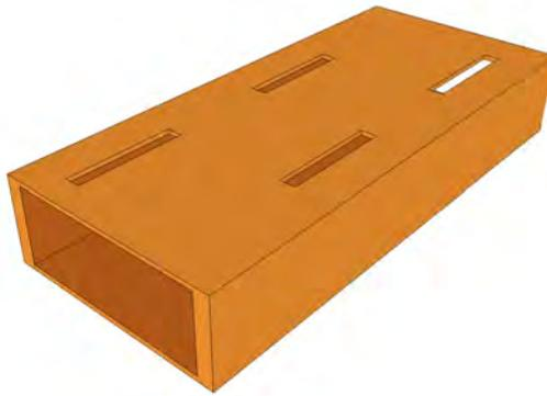
Figure 1.11: A slot waveguide antenna.
