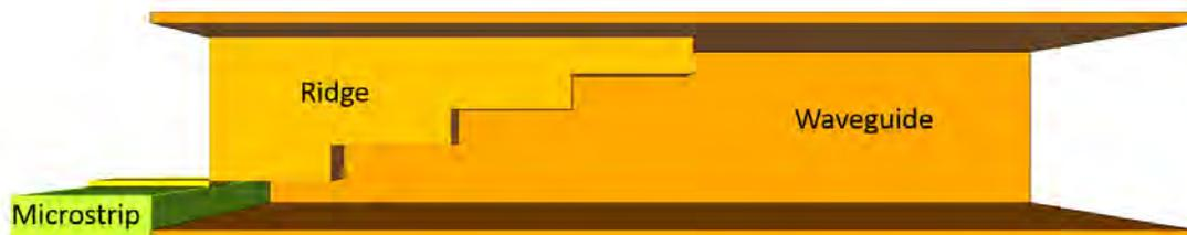
Figure 1.7: Schematic cross-section view of a ridge-to-microstrip junction
