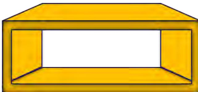
Figure 1.3: Image of a rectangular waveguide.
