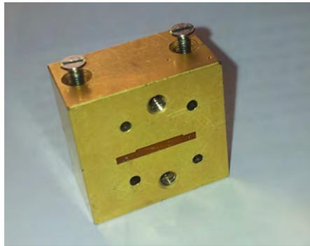
Figure 4.31: The measurement fixture for the groove gap waveguide, where the PEC metal lid is incorporated in the top part of the fixture.
