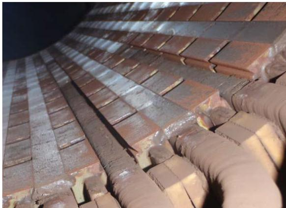
Figure 2.5 A picture of a stator missing some slot wedges, presented in [20].
