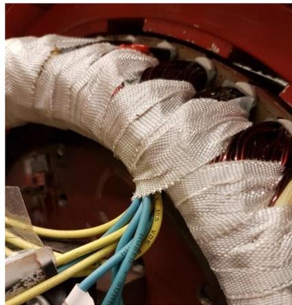
Figure 7.2 Figure a presents a schematic representation of the additional conductors and figure b presents a photo of the additional conductors added to the winding.
