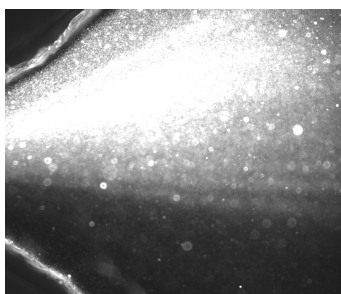
Figure 5.2: Result for the mixing through the use of a T connector to generate turbulence.
