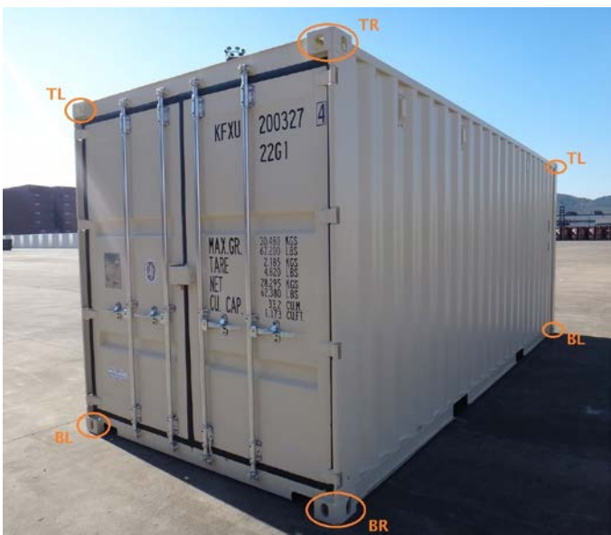
Figure 3 corner castings on a container (Chassis King, 2016)
