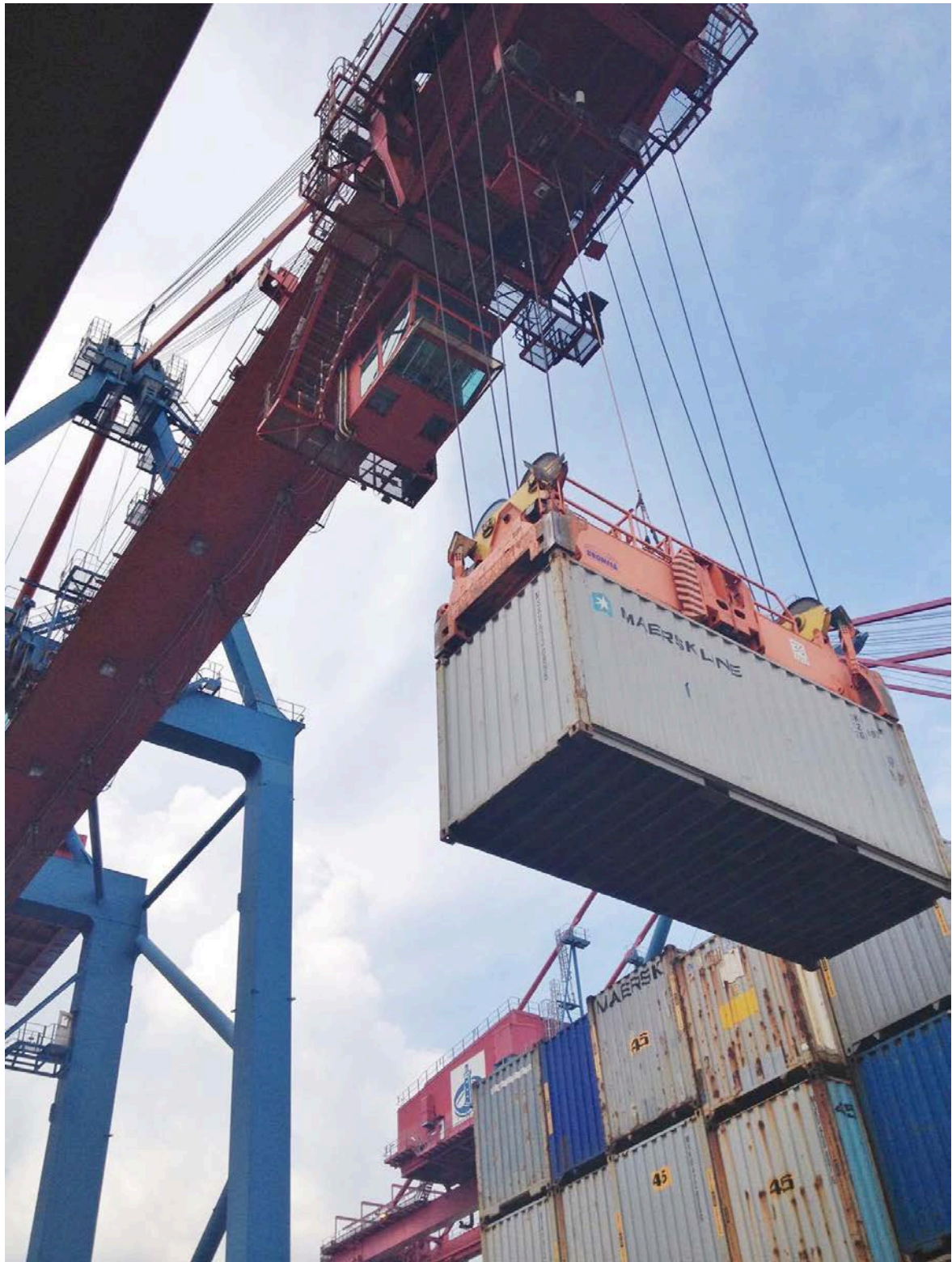
Figure 8 crane cabin and spreader (Johansson, N, 2015)
