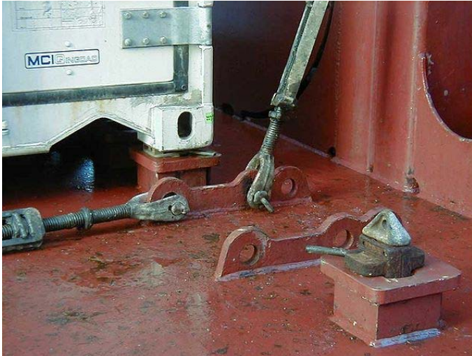
Figure 1 manually locked twist lock on deck (Wikipedia, 2016)
