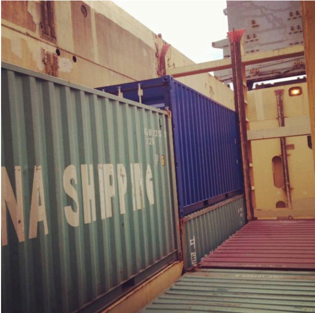
Figure 4 cell guides with insertion guides (Johansson. N, 2015)
