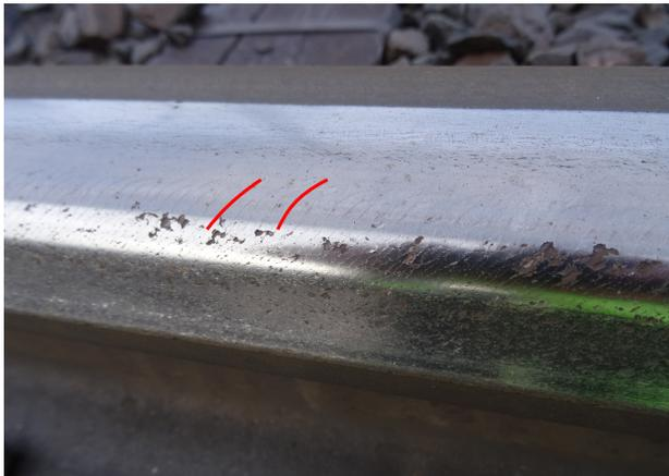
Figure 1.1: *Periodic formation of RCF cracks at the gauge corner of a railway track.*
