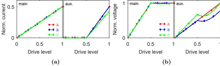
**Figure 4.11:** (a) Current and (b) voltage profiles of the generalized Doherty PA for Case A, B and C. The current is normalized with  $I_{MAX}$ . The voltage is normalized with  $V_{DS}$ .
