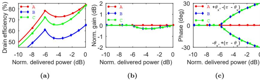
**Figure 4.13:** (a) Drain efficiency, (b) gain, and (c) phase versus normalized delivered power of the Doherty PA, for the generalized Doherty PA for Case A, B and C. The gain is normalized with itself.
