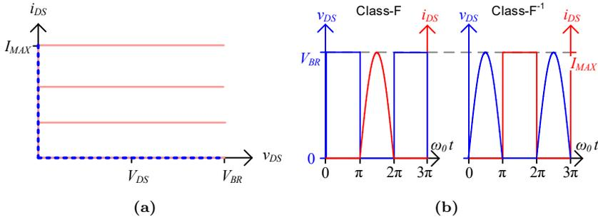
**Figure 2.9:** (a) Load line of a switch-mode PA and (b) the waveforms of class-F/-F<sup>-1</sup>.
