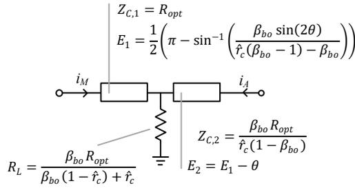
**Figure 4.6:** One combiner solution to the generalized Doherty PA architecture when  $\theta = +\theta_x$ .
