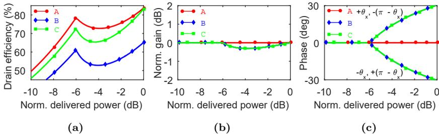
**Figure 4.13:** (a) Drain efficiency, (b) gain, and (c) phase versus normalized delivered power of the Doherty PA, for the generalized Doherty PA for Case A, B and C. The gain is normalized with itself.
