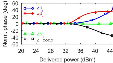
**Figure 4.15:** The phase response in different planes for cut-ready simulations.
