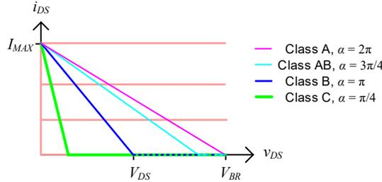
**Figure 2.5:** Load lines on top of IV-curves for class-A, AB, B, and C at maximum drive level ( $\beta = 1$ ). Class-AB and -C are continuums of conduction angles but are represented with fixed values in the figure.
