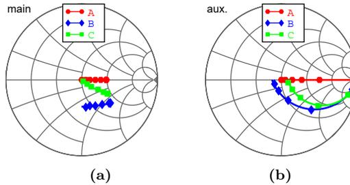
**Figure 4.12:** (a) Main and (b) auxiliary transistor load modulation versus delivered power for the generalized Doherty PA for Case A, B and C. The load is normalized with the optimum class-B load in both plots. The load modulation is valid for  $\theta = +\theta_x$  and  $\theta = -(\pi - \theta_x)$  and negative  $X_m$ .
