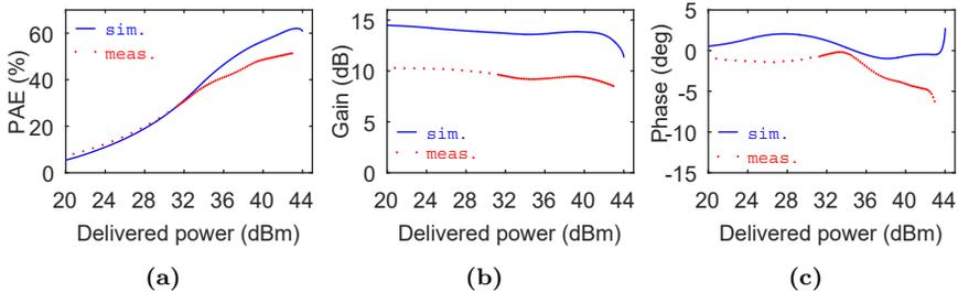
**Figure 4.16:** (a) Drain efficiency, (b) gain, and (c) phase versus delivered power for cut-ready simulations and measurements.
