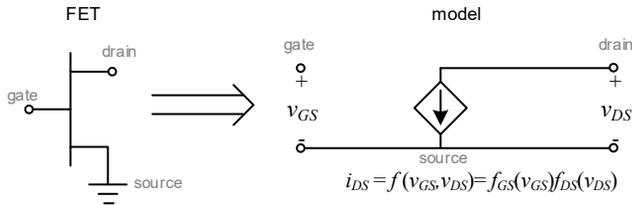
**Figure 2.1:** A FET can be modelled with a piece-wise linear current source.
