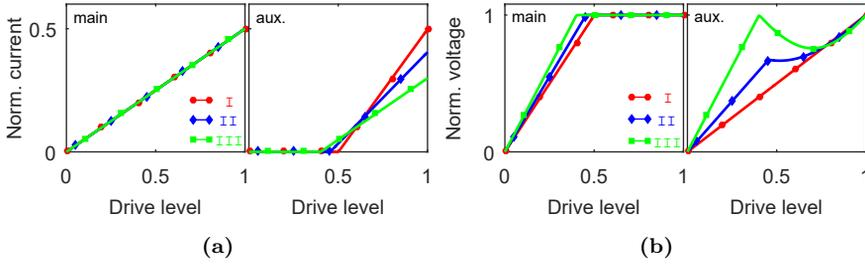
**Figure 4.8:** (a) Current and (b) voltage profiles of the generalized Doherty PA for Case I, II and III. The current is normalized with  $I_{MAX}$ . The voltage is normalized with  $V_{DS}$ .
