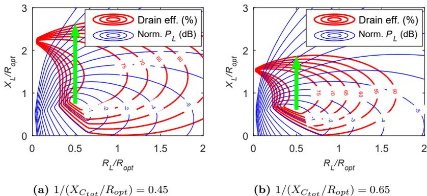
**Figure 3.3:** Drain efficiency and delivered power versus the resistive and reactive parts of the load termination, for two different  $1/(X_{C_{tot}}/R_{opt})$ . The green arrow shows a possible purely reactive load modulation.
