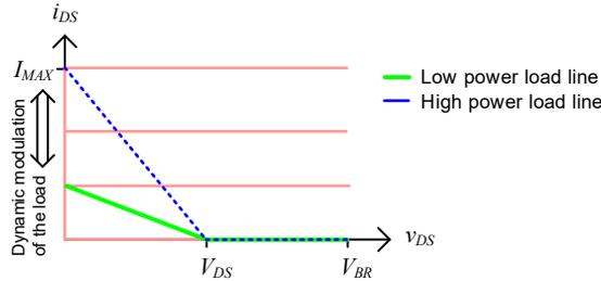
**Figure 2.11:** Load lines for load modulation. The fundamental load termination resistance is modulated dynamically as an inverse function of the drive level.
