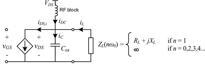
**Figure 3.2:** Schematic of class-J operation.
