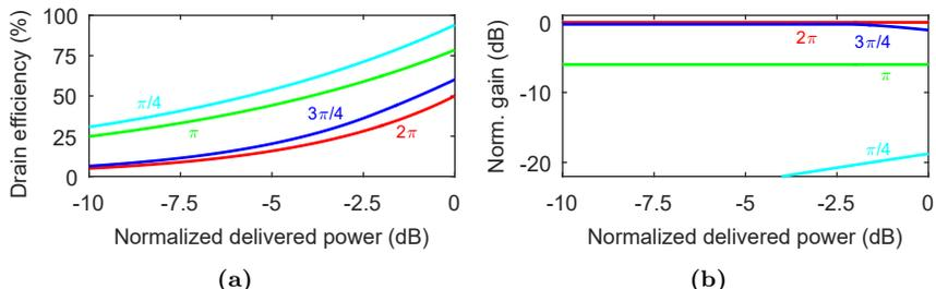
**Figure 2.8:** PA characteristics versus delivered power for class-A ( $\alpha = 2\pi$ ), -AB ( $\alpha = 3\pi/4$ ), -B ( $\alpha = \pi$ ) and -C ( $\alpha = \pi/4$ ). (a) Presents drain efficiency and (b) presents gain normalized with the class-A gain. The delivered powers are normalized with their maximum value.
