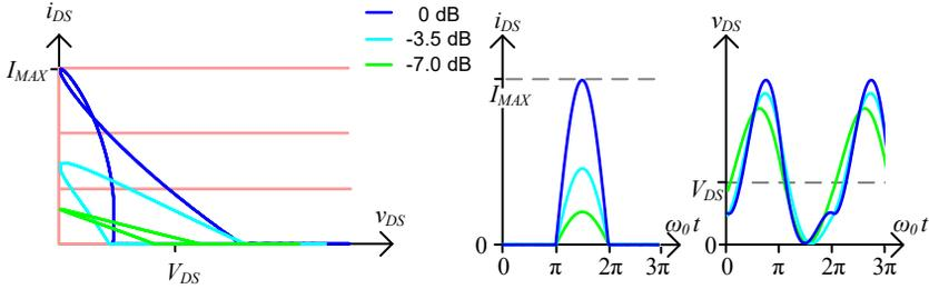
**Figure 3.6:** Load lines and waveforms for a purely reactive load modulated class-J PA with  $1/(X_{C_{tot}}/R_{opt}) = 0.55$  and  $R_L/R_{opt} = 0.5$ , for different normalized delivered powers.
