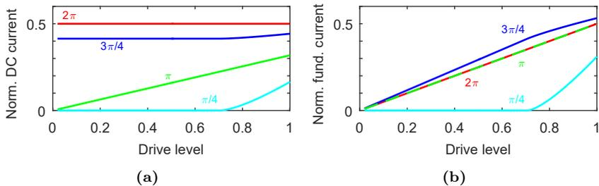
**Figure 2.7:** PA characteristics versus drive level for class-A ( $\alpha = 2\pi$ ), -AB ( $\alpha = 3\pi/4$ ), -B ( $\alpha = \pi$ ) and -C ( $\alpha = \pi/4$ ). (a) Presents DC currents and (b) presents fundamental currents, all normalized with  $I_{MAX}$ .
