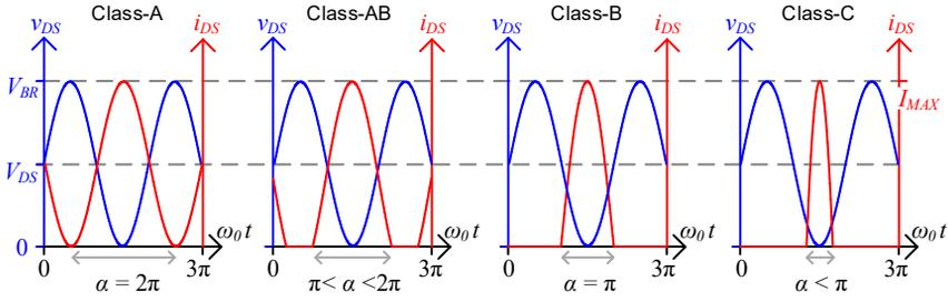
**Figure 2.4:** The voltage and current waveforms for the amplifier classes A, AB, B and C, at the drive level  $\beta = 1$ . All have a purely sinusoidal voltage waveform but differ by the conduction angle,  $\alpha$ , of the current waveform.
