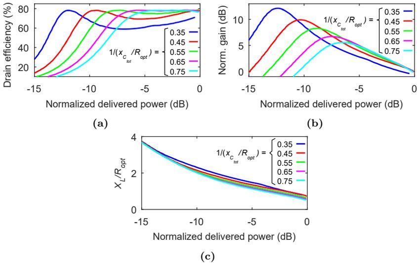
**Figure 3.5:** Cross sections for different  $1/(X_{C_{tot}}/R_{opt})$ , for a fixed  $R_L/R_{opt} = 0.5$ .
