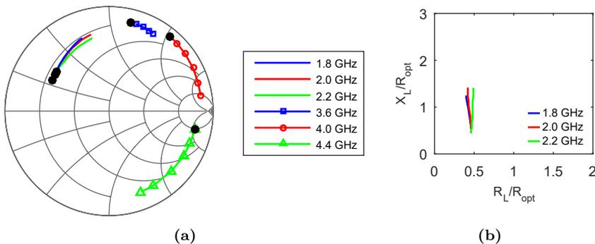
**Figure 3.11:** (a) Fundamental and second harmonic load modulation for cut-ready simulations, represented by reflection coefficients in a Smith chart normalized with  $50 \Omega$ . The maximum power levels are marked with a solid black circle. (b) Fundamental load modulation for cut-ready simulations in Cartesian coordinates normalized with  $R_{opt} = 27 \Omega$ .
