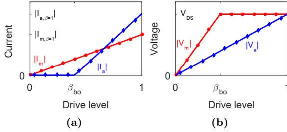
**Figure 4.2:** (a) Current and (b) voltage profiles of the conventional Doherty PA.
