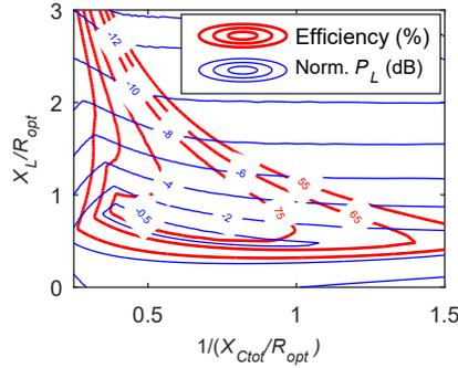
**Figure 3.4:** Drain efficiency and delivered power versus the reactive part of the load termination and  $1/(X_{C_{tot}}/R_{opt})$  (proportional to frequency), for a fixed  $R_L/R_{opt} = 0.5$ .
