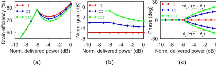
**Figure 4.10:** (a) Drain efficiency, (b) gain, and (c) phase versus normalized delivered power of the Doherty PA, for the generalized Doherty PA for Case I, II and III. The gain is normalized with the single class-B gain.
