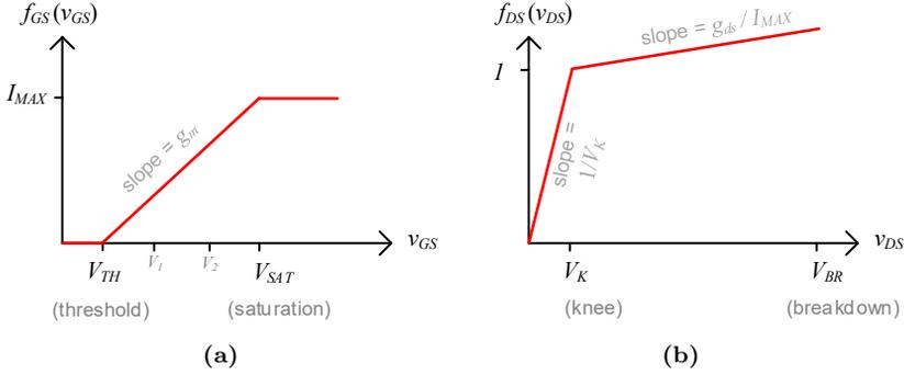
**Figure 2.2:** The separated functions in a piece-wise linear current source.
