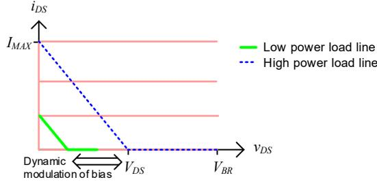
**Figure 2.10:** Load lines for supply modulation. The drain bias is modulated dynamically as a function of the drive level.
