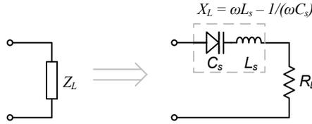
**Figure 3.7:** A series varactor and series inductor configuration for achieving a purely reactive load modulation.
