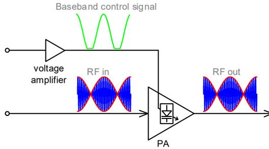
**Figure 3.1:** Varactor-based dynamic load modulation architecture.
