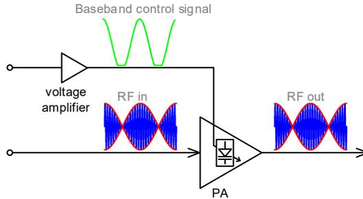
**Figure 3.1:** Varactor-based dynamic load modulation architecture.
