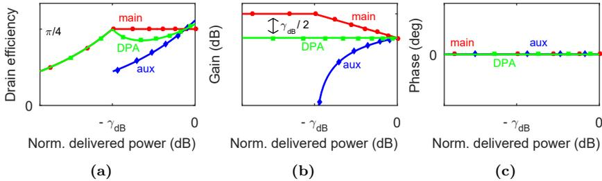
**Figure 4.4:** (a) Drain efficiency, (b) gain, and (c) phase of the main transistor, the auxiliary transistor, and the Doherty PA, versus normalized delivered power of the Doherty PA.
