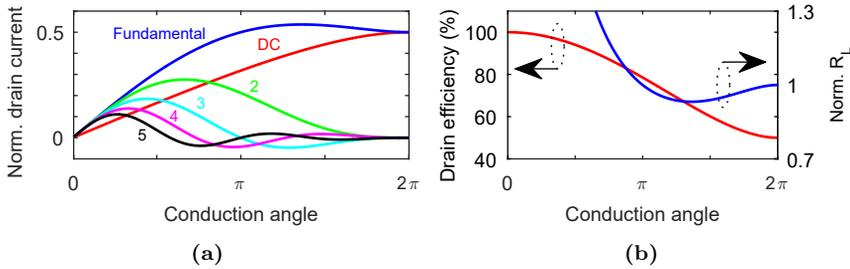
**Figure 2.6:** PA characteristics versus conduction angle when  $\beta = 1$ . (a) Presents normalized DC- and five first harmonic frequency components of the drain current, and (b) presents drain efficiency and normalized fundamental load termination  $R_L$ . The frequency components are normalized with  $I_{MAX}$ .  $R_L$  is normalized with the class-A fundamental load termination.
