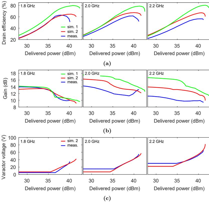
**Figure 3.10:** (a) Drain efficiency, (b) gain, and (c) varactor voltage versus delivered power for 1.8, 2.0 and 2.2 GHz. *Sim. 1* denotes simulations with a real transistor model and ideal input/output networks, *sim. 2* denotes cut-ready simulations, and *meas.* denotes measurements of the fabricated prototype.
