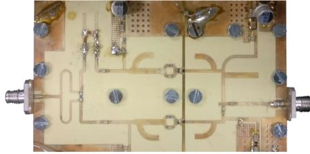
**Figure 4.14:** Photograph of the core area of the fabricated Doherty PA. The transistors are soldered to a ridge in the middle.
