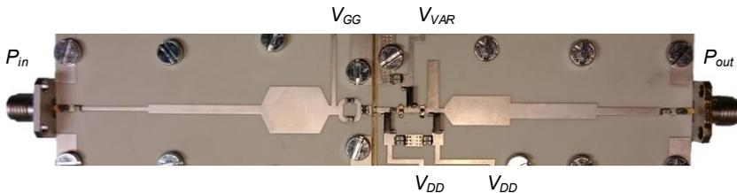
**Figure 3.8:** Photograph of the core area of the fabricated varactor-based DLM PA. The transistor is soldered to a ridge in the middle.
