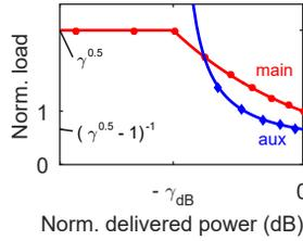
**Figure 4.3:** The main and auxiliary transistor load modulation versus normalized delivered power of the Doherty PA, for the conventional Doherty PA. The load is normalized with the optimum class-B load.
