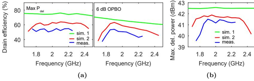
**Figure 3.9:** (a) Drain efficiency versus frequency at maximum delivered power and at 6 dB OPBO. (b) Maximum delivered power versus frequency. *Sim. 1* denotes simulations with a real transistor model and ideal input/output networks, *sim. 2* denotes cut-ready simulations, and *meas.* denotes measurements of the fabricated prototype.
