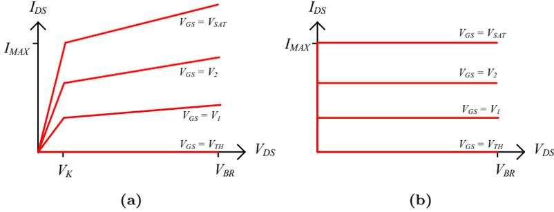
**Figure 2.3:** The DC-characteristics of (a) a piece-wise linear current source and (b) a piece-wise linear current source with  $g_{ds} = 0$  and  $V_K = 0$ .
