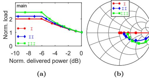
**Figure 4.9:** (a) Main and (b) auxiliary transistor load modulation versus delivered power for the generalized Doherty PA for Case I, II and III. The load is normalized with the optimum class-B load in both plots. The load modulation of the main transistor is purely resistive and is therefore shown in a Cartesian plot. The load modulation in (b) is valid for  $\theta = +\theta_x$  and  $\theta = -(\pi - \theta_x)$ .
